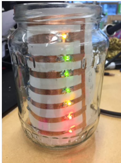
Fig. 3. Labwork: Prototype of an LED node with paper and copper tape.
